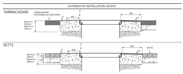
1.2m eight sided solid base sump, corbel, height skirt adjustable, internal lid, 900mm dia. watertight flat sealed cover and frame.
