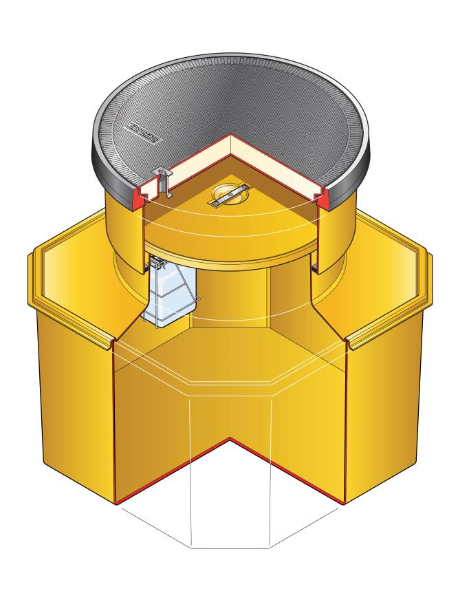
1.2m eight sided solid base sump, corbel, height skirt adjustable, internal lid, 900mm dia. watertight flat sealed cover and frame.
