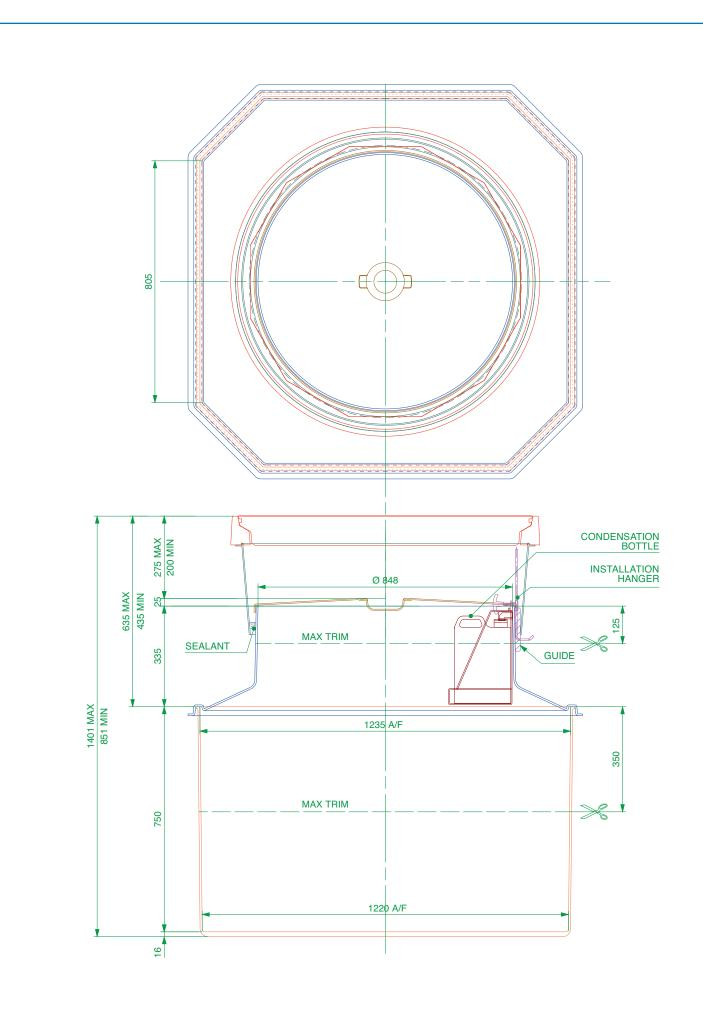
1.2m eight sided solid base sump, corbel, height skirt adjustable, internal lid, 900mm dia. waterlight flat sealed cover and frame.
