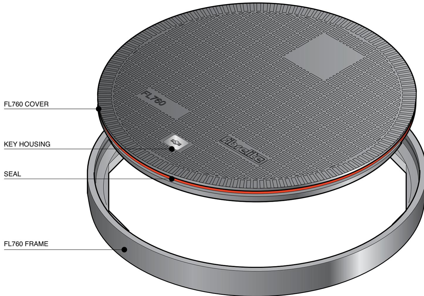
762 diameter flat sealed composite cover and frame.
