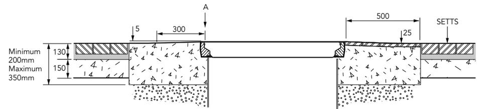
762 diameter flat sealed composite cover and frame.
