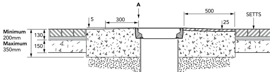
300mm diameter flat sealed composite cover and frame.
