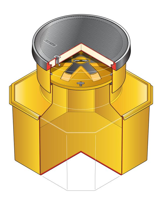
1.2m eight sided solid base chamber, corbel, adjustable height skirt, watertight internal platform, 900mm dia. watertight flat sealed cover and frame.
