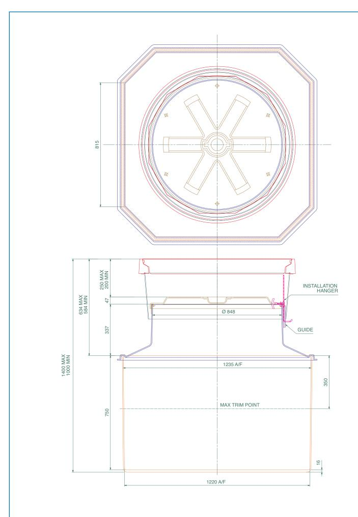
1.2m eight sided solid base chamber, corbel, adjustable height skirt, watertight internal platform, 900mm dia. watertight flat sealed cover and frame.
