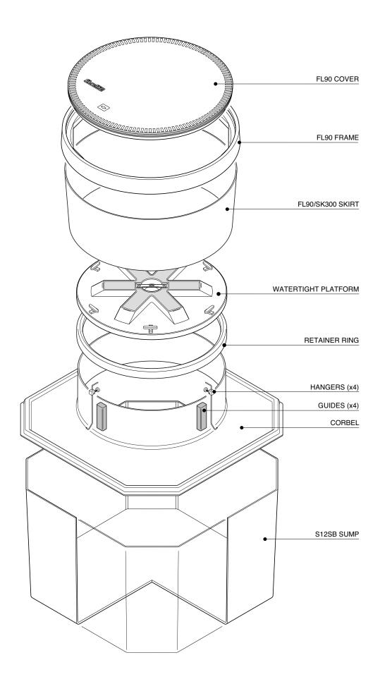
1.2m eight sided solid base chamber, corbel, adjustable height skirt, watertight internal platform, 900mm dia. watertight flat sealed cover and frame.
