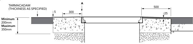
900mm dia. watertight flat sealed composite cover and frame, with a central dip port cover.
