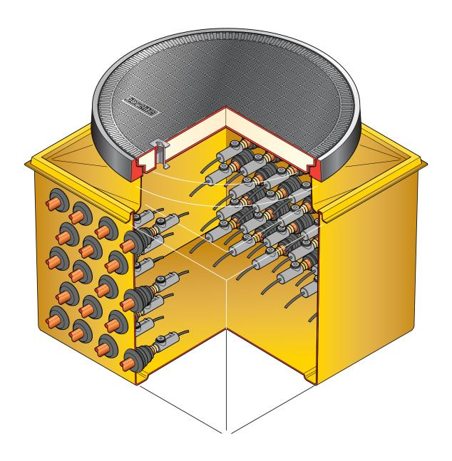
$862\text{mm} \times 862\text{mm} \times 675\text{mm}$  deep solid base sump with a corbel and 760mm dia. flat sealed cover and frame.
