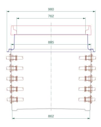
$862\text{mm} \times 862\text{mm} \times 675\text{mm}$  deep solid base sump with a corbel and 760mm dia. flat sealed cover and frame.
