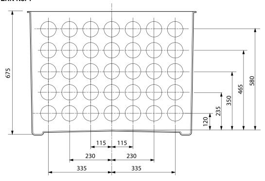
$862\text{mm} \times 862\text{mm} \times 675\text{mm}$  deep solid base sump with a corbel and 760mm dia. flat sealed cover and frame.
