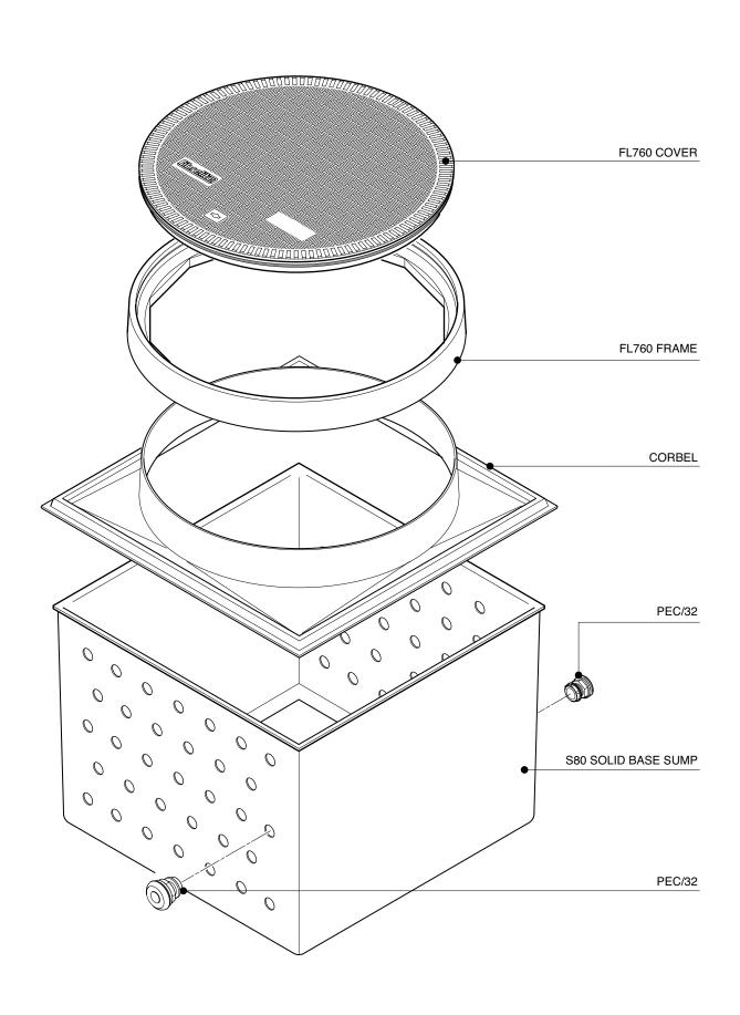
$862\text{mm} \times 862\text{mm} \times 675\text{mm}$  deep solid base sump with a corbel and 760mm dia. flat sealed cover and frame.
