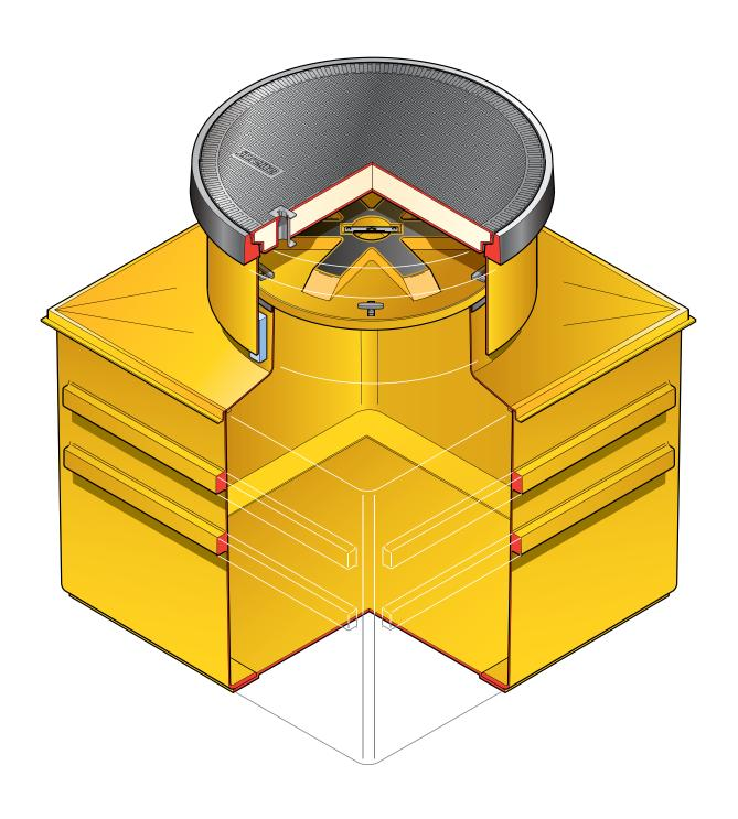
1.2m square solid base chamber with a sealed corbel, adjustable skirt, internal watertight platform and round 900mm flat sealed cover.
