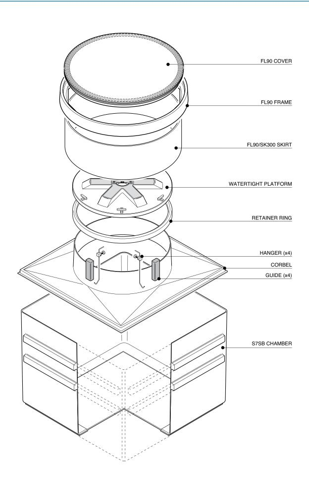
1.2m square solid base chamber with a sealed corbel, adjustable skirt, internal watertight platform and round 900mm flat sealed cover.
