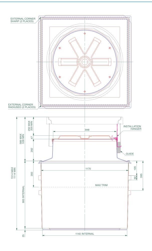
1.2m square solid base chamber with a sealed corbel, adjustable skirt, internal watertight platform and round 900mm flat sealed cover.
