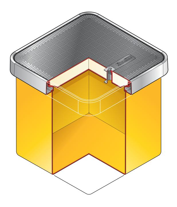
$600\mbox{mm}$  square x  $600\mbox{mm}$  deep solid base chamber with a square  $600\mbox{mm}$  flat sealed cover.
