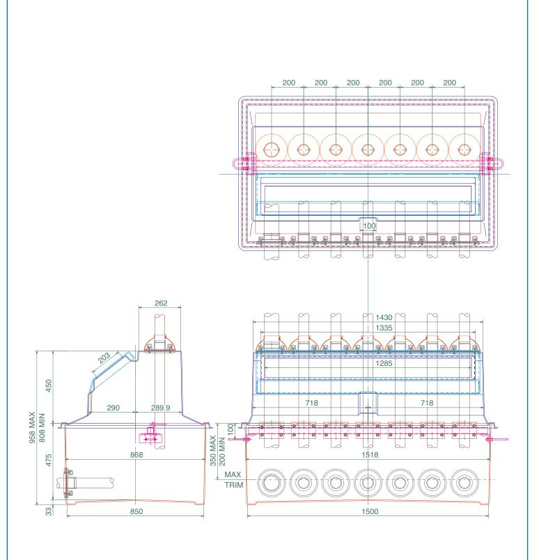
Vent pipe transition sump. 1500mm x 850mm x 475mm below ground solid base sump, with 450mm high above ground sealed top with lockable hinged door. Includes pipework support rail and fixings. Order pipe entry boots PSB/63, PSB/90 PSB/63/VT, PSB/90/VT & vent riser mounting brackets MPK-VENT separately.
