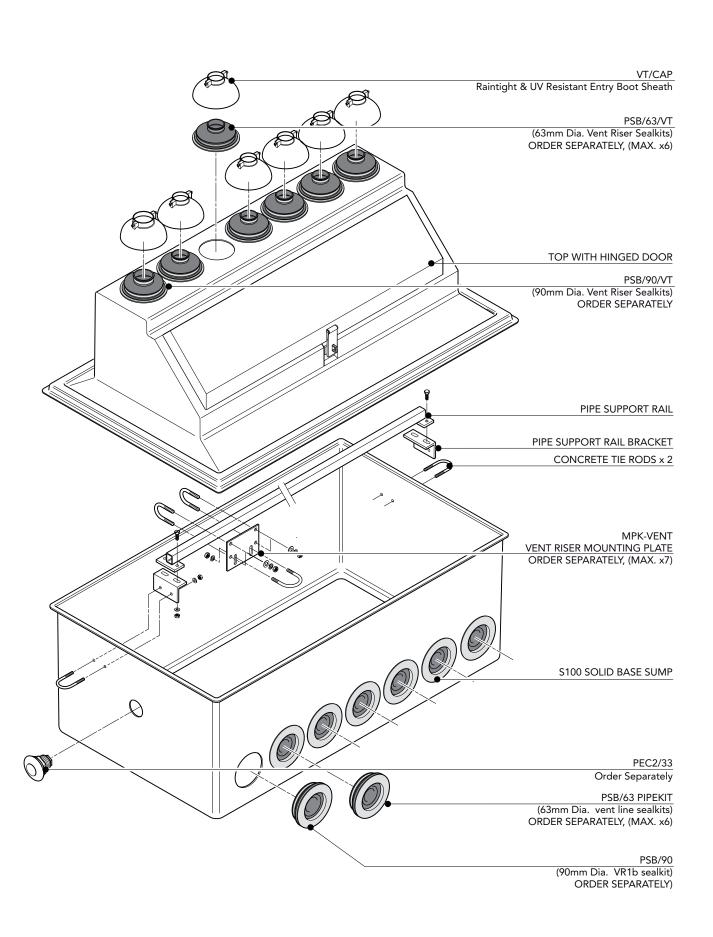
Vent pipe transition sump. 1500mm x 850mm x 475mm below ground solid base sump, with 450mm high above ground sealed top with lockable hinged door. Includes pipework support rail and fixings. Order pipe entry boots PSB/63, PSB/90 PSB/63/VT, PSB/90/VT & vent riser mounting brackets MPK-VENT separately.
