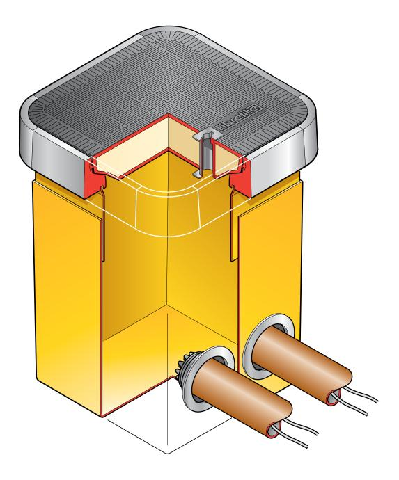
Electrical Drawpit 450mm square x 600mm GRP base chamber with a  $\,$  210mm deep skirt and square 450mm flat sealed cover.
