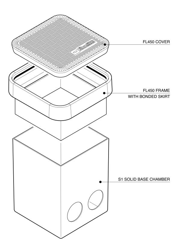
Electrical Drawpit 450mm square x 600mm GRP base chamber with a  $\,$  210mm deep skirt and square 450mm flat sealed cover.
