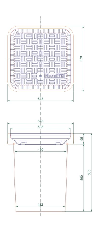
450mm square x 600mm deep solid base chamber with a square 450mm flat sealed cover and frame.
