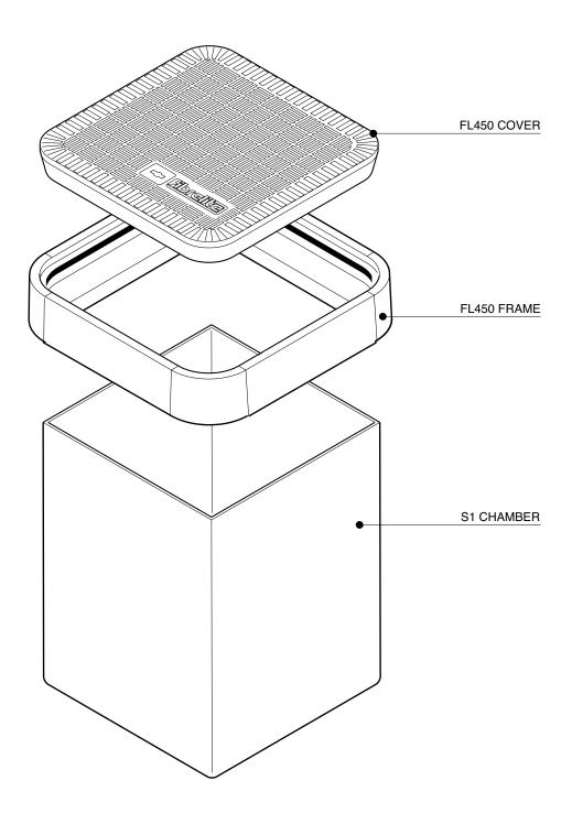
$450 \mathrm{mm}$  square x  $600 \mathrm{mm}$  deep solid base chamber with a square  $450 \mathrm{mm}$  flat sealed cover and frame.
