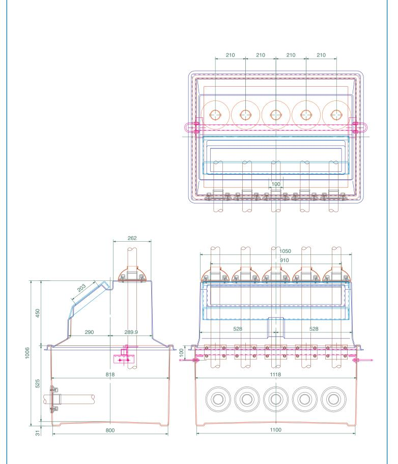
Vent pipe transition sump. 1100mm x 800mm x 525mm below ground solid base sump, with 450mm high above ground sealed top with lockable hinged door. Includes pipework support rail and fixings. Order pipe entry boots PSB/75, PSB/63/VT & vent riser mounting brackets MPK-VENT separately.
