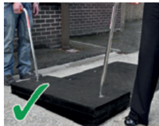
Safe lifting technique with Fibrelite Lifting aid
