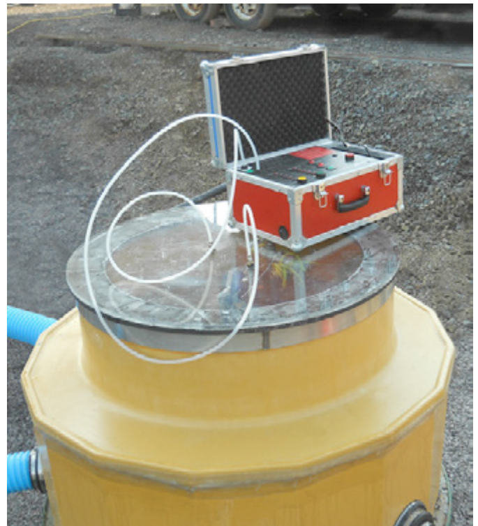
Vacuum testing to ensure a watertight installation
