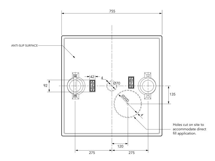
Solid structural platform with hole markings for a offset direct fill and central dipstick. Fits square chamber systems with a FL76 cover. Holes cut on site. Anti-slip surface.
