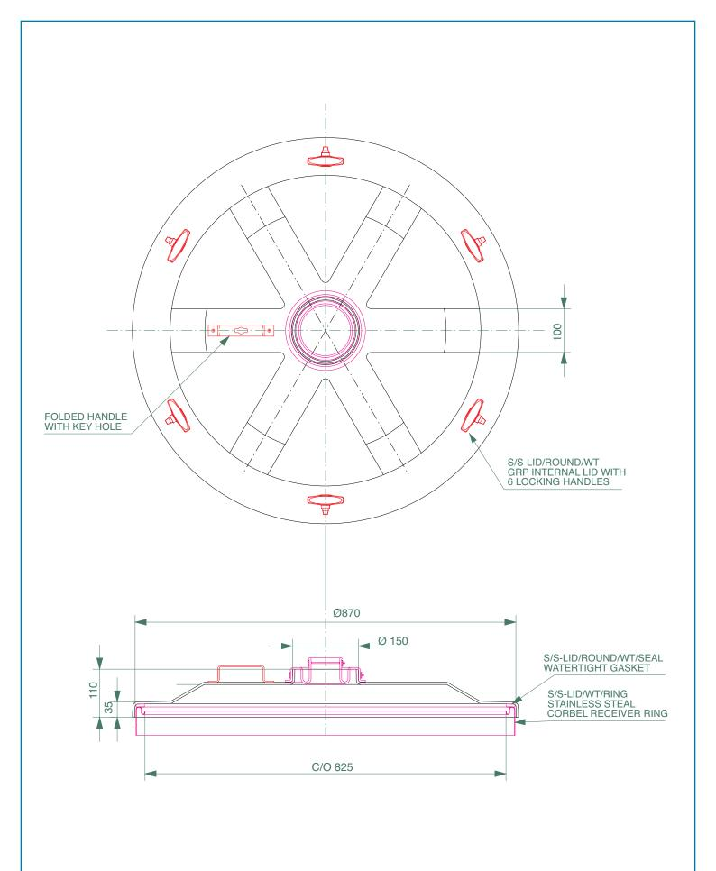
Watertight lock-down internal lid to fit chamber systems with a FL90 cover. Connects to stainless steel corbel ring (S/S-LID/WT/RING).
