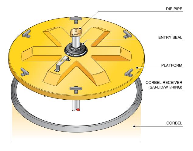
Watertight lock-down internal lid to fit chamber systems with a FL90 cover. Connects to stainless steel corbel ring (S/S-LID/WT/RING).
