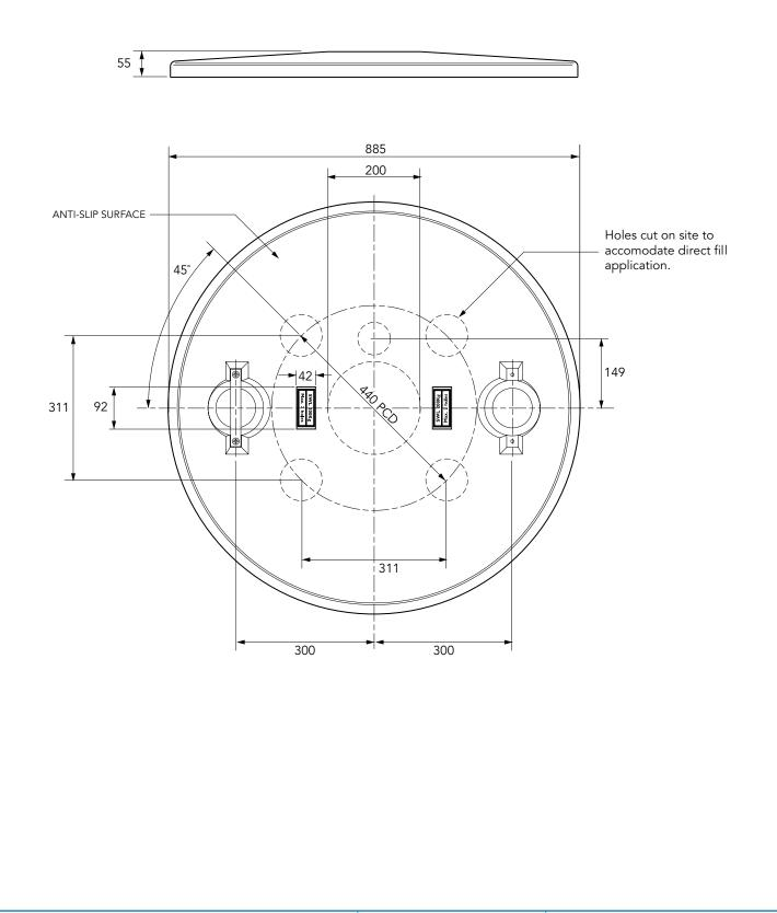
Solid structural platform with hole markings for central fill (20cm dia) and offset dip positions. Fits all chambers systems with FL90 cover. Cut holes on site. Anti-slip surface.
