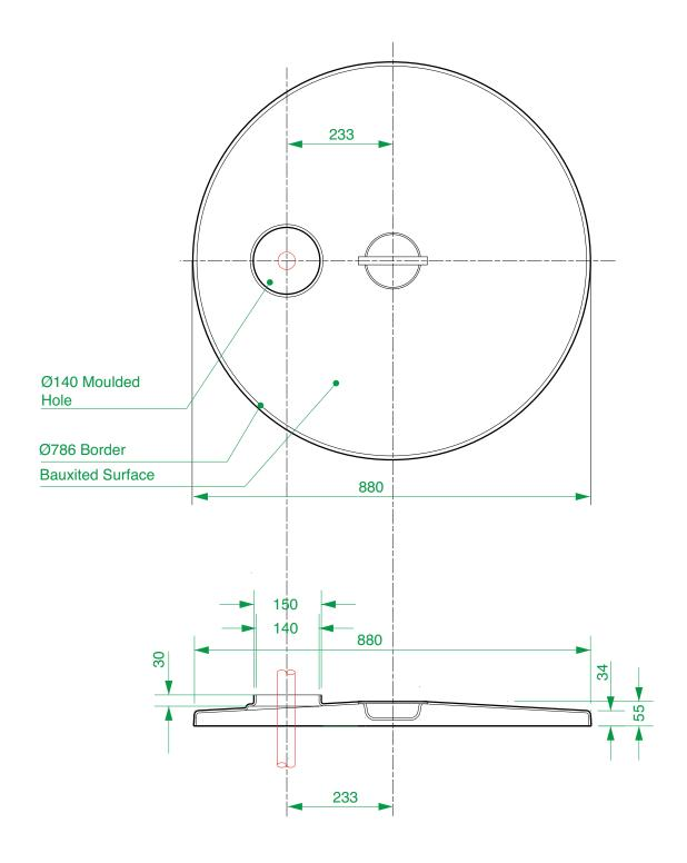
Structural platform with moulded offset sealed port for manual dip stick. Fits all chamber systems with FL90 cover. Anti-slip surface.
