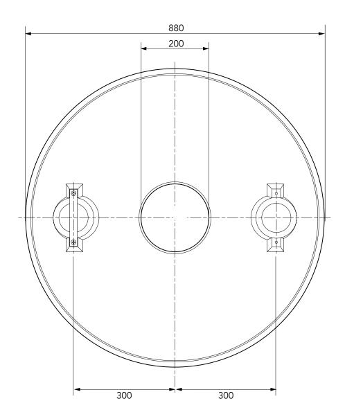
Non structural internal lid, with central manual dip hole (20cm). Fits all chamber systems with FL90 cover.
