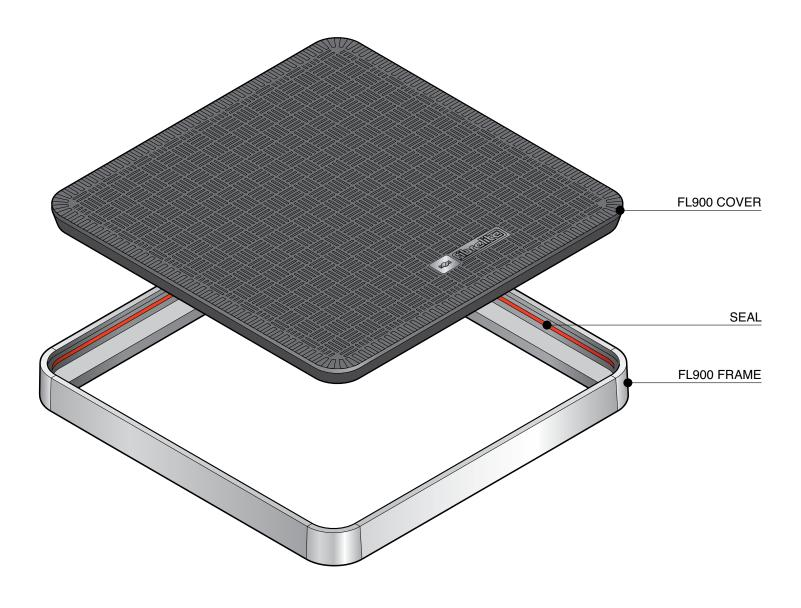
900mm square flat sealed composite cover with an aluminum frame.
