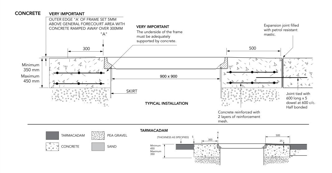
900mm square flat sealed composite cover with an aluminum frame.
