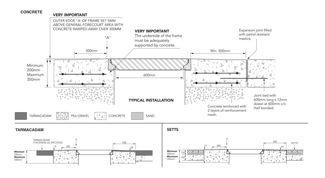
600mm x 600mm flat sealed composite cover with an aluminium frame.
